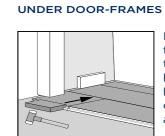
bar. Gently tap with a hammer to gradually connect the panels in a few taps.
